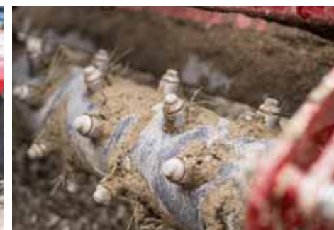
Power: 72 carbide tips pulverize the surface
