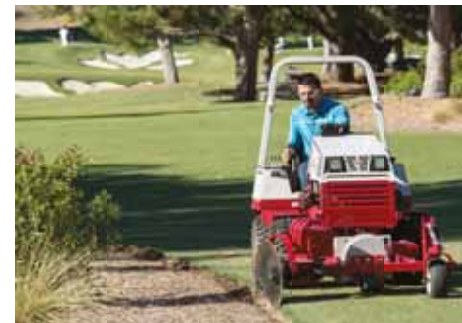
Bevel Out: Reverse Disc To Shape Beds
