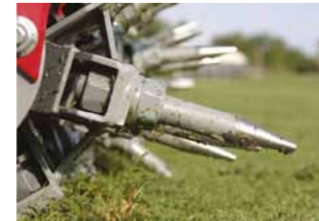
Cores Turf While Loosening Soil
