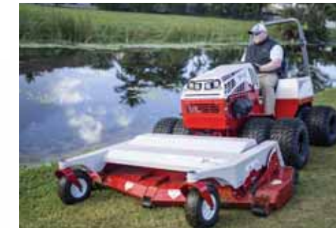
Contour following: Fully Rotating Deck
