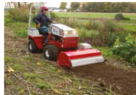
Reverse Operation for Undisturbed Tilled Areas
