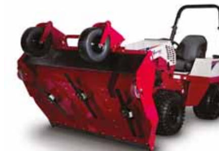
Easy Maintenance: Tilt-Up Deck
